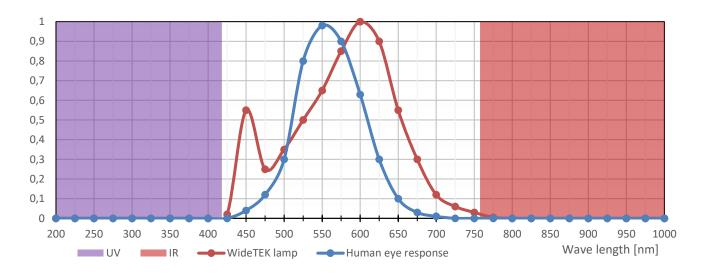
The radiated spectrum of the white LED lights on a WideTEK or Bookeye scanner is between 420 and 760 nm. This is completely inside the visible spectrum of the human eye. There is no unintended emission of UV light (purple area at the left side of the diagram) and no emission of IR (red area at the right side of the diagram), only useful light is emitted (white, middle section).
