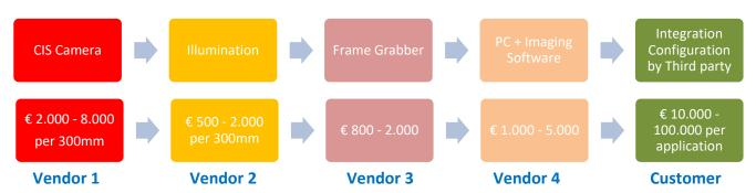
Various vendors offer CIS cameras in different width. Some of them have illumination built in, in some cases they need to be added to the bill of material. After the camera is chosen by the customer, a frame grabber is needed to get the images into a PC. Whether the interface is GigE, Camera Link or other, the cabling is significant and bulky. At the end of the process the components delivered by three or four parties have to be integrated by the customer to create the final application.
