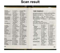
The scan result shows the content of both pages. The curvature of the book binding is flattened and the pattern at the margins has been removed.
