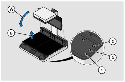
The automatic locking of the glass plate in the lowered state is switched on or off with the Cradle Lock button (4).
