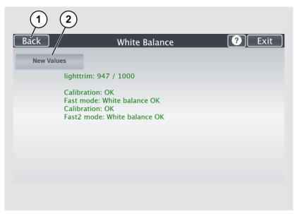
On an error-free white balance calibration, the result is displayed in green.
