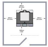
Place the Bookeye® 4 scanner on a flat and solid base. The load bearing capacity of the base must correspond to the device weight. The dimensions of the base must match the floor space required by the scanner.
