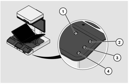
The key board of a Bookeye® 4 has, depending on the scanner model, two or more buttons with additional functions.
