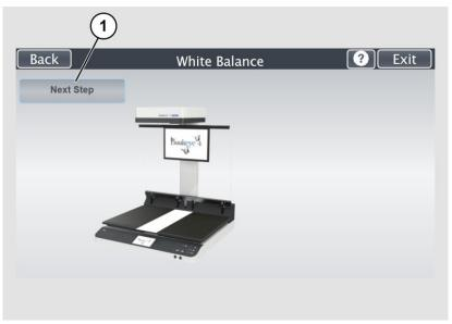
The white balance starts and the calibration is performed. During the white balance, a rotating icon appears. The entire white balance sequence takes about 40 seconds.
