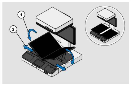
The plates can also be set to the "V" position, with an opening angle of 120 degrees. This is recommended for very delicate, old books and documents. The plates are held in position by a supporting leg on each side.
