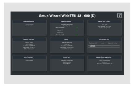
The Setup Wizard allows the user to perform the most important settings on the touch screen during the initial installation of a Scan2Net scanner. After the Setup Wizard has been successfully completed, the scanner can be used immediately without any further settings.
