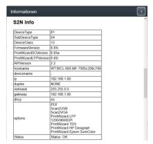
The S2N INFO section shows you detailed information about your Scan2Net hardware device, such as the device type and subtype, hardware hostname of the device, IP address, gateway address and subnet mask address, the firmware version installed, and options installed.
