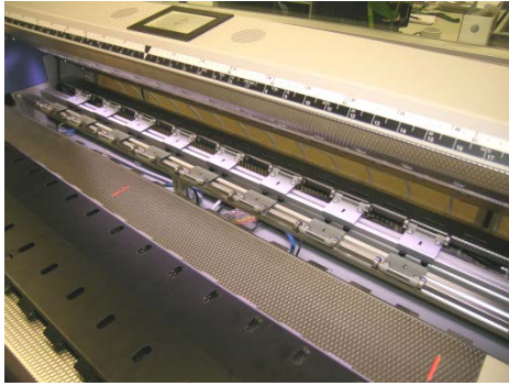
Picture 77: Compensator plate on document table
